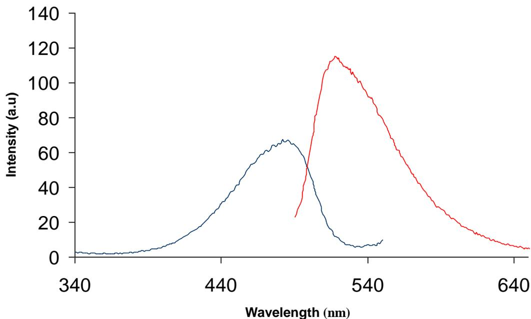
**Figure 3.** excitation (blue) and emission (red) spectrum of 10uM BO21 in water.
